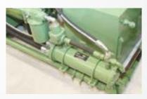
All TURBO-AIR compressors feature a self-contained, low-pressure lubrication system.
